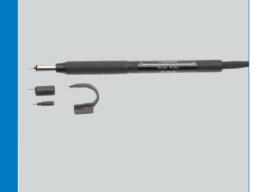
The 1205 RF Probe 20 dB is a passive 10:1 RF voltage probe with a 50 VDC block built in. It has been designed to allow users of RF test equipment to use standard signal tracing techniques. The probe makes it possible to conveniently and accurately monitor or inject signals up to 4 GHz into RF circuits without significantly loading or detuning them.
